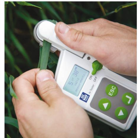
Figure 8: The Yara N-Tester is a handheld tool that provides immediate information on actual nitrogen need.
